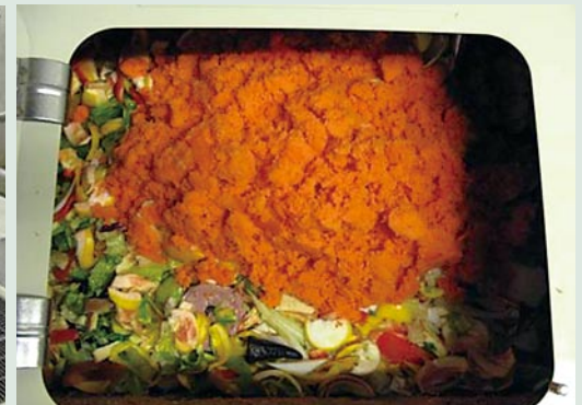
The Peninsula Tokyo introduced the 'Gomizer' machine in 2009, which converts perishable waste through a cost effective, environmentally responsible yeast/bacteria process into a liquid for safe discharge to the sewage system, thereby dispensing of more than 50 kg of waste per day. As of 1 March 2009, an estimated 15,000 kg of perishable garbage had been processed.
