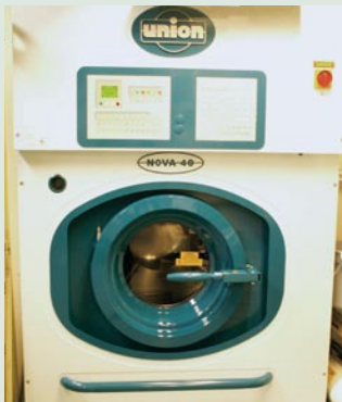
The Peninsula Chicago installed a "hydro carbon" dry cleaning machine to reduce chemical consumption.
